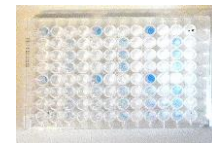
Picture 1: Typical Microfilter plate for the Elispot assay
